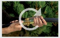
To disconnect, push the coupling and the counterpart together in axial direction. Afterwards, turn one coupling half as far as possible in the opposite direction as you would do when connecting and remove it from the counterpart.
