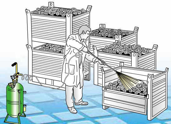
Spraying antioxidant, oil, diesel oil on mechanical parts
