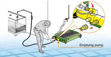
The drained oil can be transferred from the collection bowl to the storage tank by suction with the incorporated probe or by an emptying pump connected to the fixed system or mounted directly on the collection basin
