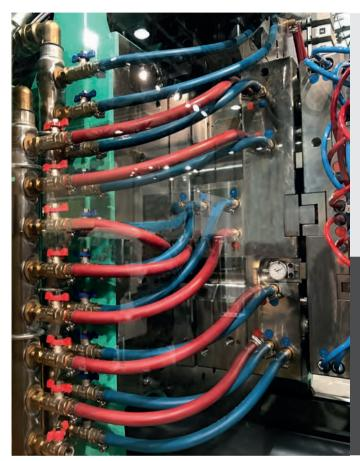
Plastic processing companies rely on particularly robust and sturdy couplings and fittings. The reason: They are used to cool and heat moulding units during injection moulding or pressure casting and have to withstand extreme temperatures.
