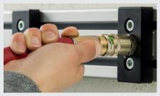
Coupling with one-hand operation - To connect the system, simply push the plug into the safety coupling. The release sleeve automatically slides forward in a twisting motion and engages into the final safety lock position.
