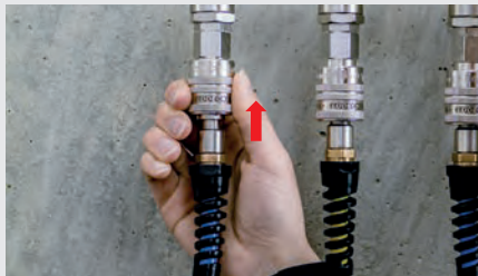
Disconnection - first step: Automatic venting
