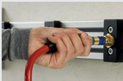
One-hand operation: To connect, push the plug into the coupling. (The colours of the aluminium sleeve of the coupling and the aluminium ring of the plug as well as the plug-coding have to be identical.)
