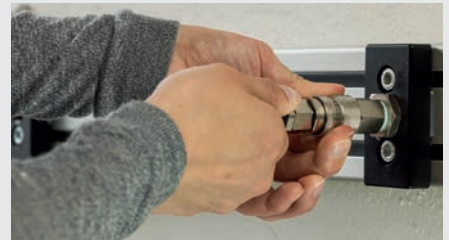
Two-hand operation: To disconnect, push the plug while pulling back the sleeve
