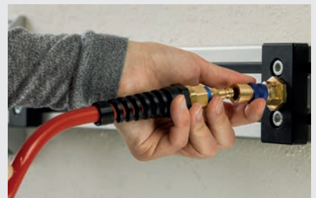
To disconnect, pull back the coupling sleeve.
