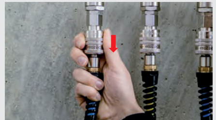
Disconnection - second step: Safe decoupling
