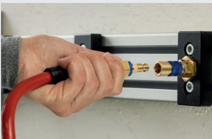
One-hand operation: To connect, push the plug into the coupling. (The colours of the aluminium sleeve of the coupling and the aluminium ring of the plug as well as the plug-coding have to be identical.)
