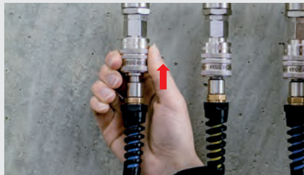
Disconnection - first step: Automatic venting
