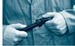
Step 3: Pull the corrugated tube back slightly inside the connector (to latch securely).
