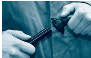
Step 5: Pull the corrugated tube out of the connector.
