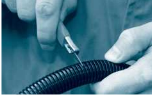
Step 1: Separate the tube at a corrugation crest (optimal protection of the tube and connector).
