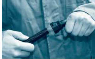
Step 2: Insert the tube into the „closed“ connector as far as it will go (to assemble the connector).
