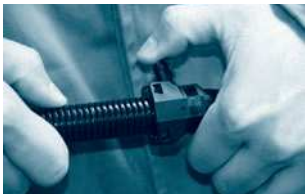
Step 4: Move the detent lugs out (to dismantle the connector).
