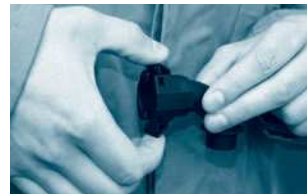
Step 6: Push the detent lugs in (NORDUC® assembly system ready to use again).
